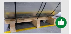
The coil is protected with foil and strapped with PE band.
