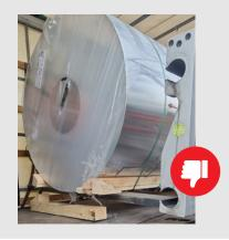
The coil mold is not protected with cardboard or foil, resulting in surface damage at unloading.
