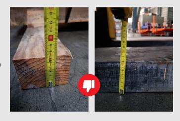
These wooden feet are higher than 8cm (very good for forklift handling) and are not wider than the material.
