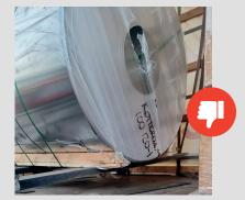
The coil mold is not protected with cardboard or foil, resulting at surface damage at unloading.
