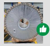
The coil edges are protected with cardboard. The mold is covered with cardboard to avoid scratches. Foil is protecting against staining/scratches.
