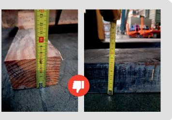
These wooden feet are higher than 10cm (very good for forklift handling) and are not wider than the material.
