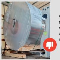
Wood must be placed under material to avoid direct lifting of material.
