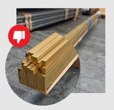
This colli has wooden feet >8cm for easy handling, the material is secured with steel band against uncontrolled movement and the top side is protected with wood.
