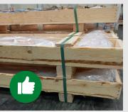
The profiles have been wrapped in plastic and are protected by wood along the entire length of the package.
