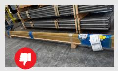
The PE/steel band on this colli has not been **mechanically tightened (!)** with a ratchet. The *"hand tight"* band got loose, resulting in the material stack falling apart.
