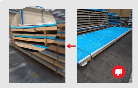
Only four wooden feet have been used, resulting in the material bending and the pallet bursting. Most common for smaller material thicknesses (<4mm)
